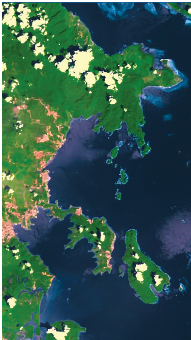
Fig. 3 - Satellite image of laterite open-pit mines -reddish areas- on Sulawesi Island (Indonesia) in 2019 (courtesy of NASA/METI/AIST/Japan Space Systems and U.S./Japan ASTER Science Team)
