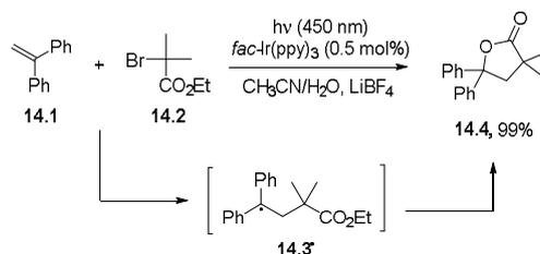
**Scheme 14.** Intermolecular addition of  $\alpha$ -bromoesters to styrenes for the photocatalyzed synthesis of  $\gamma$ -lactones.
