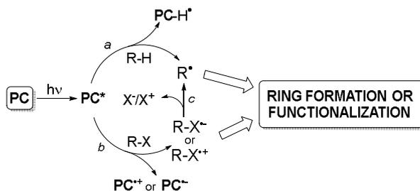
**Scheme 1.** Main pathways for the preparation of heterocycles by a photocatalytic approach (**PC**=photocatalyst).
