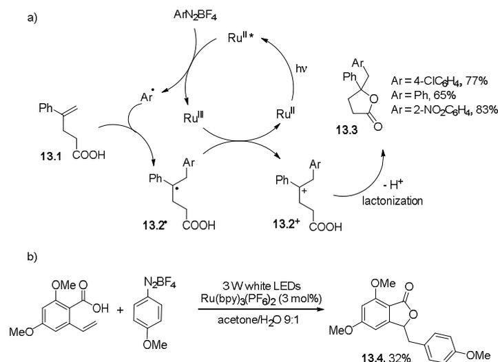
**Scheme 13.** a) Photocatalytic arylation/lactonization sequence for the synthesis of sterically hindered  $\gamma,\gamma$ -disubstituted butyrolactones and b) application of this protocol to the synthesis of the naturally-occurring compound **13.4**.
