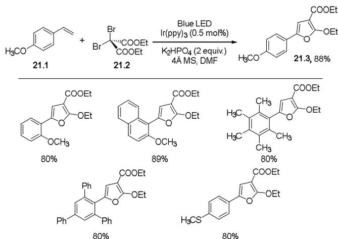
**Scheme 21.** Photocatalytic 1,2-difunctionalization of styrenes for the synthesis of furans.
