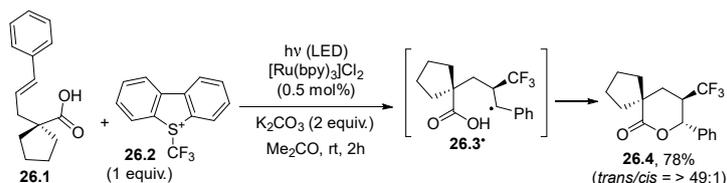
**Scheme 26.** Photocatalyzed carbolactonization of alkenoic acid **26.1**.
