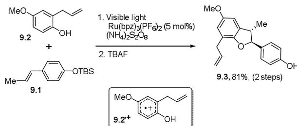
**Scheme 9.** Photocatalyzed [3+2]-cycloaddition reaction as a tool for the synthesis of 2,3-dihydrobenzofurans.
