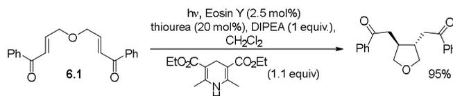
**Scheme 6.** Bis-enones as starting materials for the construction of the tetrahydrofuran ring.
