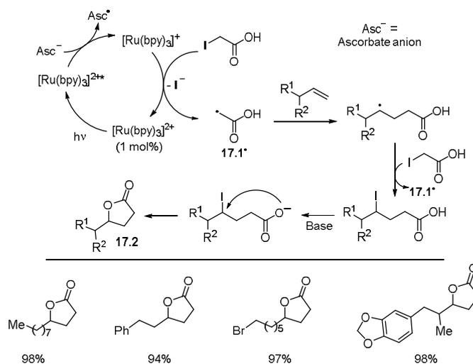
**Scheme 17.** Photocatalytic ATRA reaction for the synthesis of  $\gamma$ -lactones.
