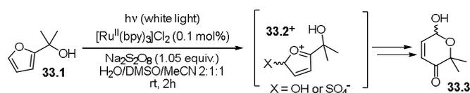
**Scheme 33.** Preparation of the 2*H*-pyran-3(6*H*)-one core.
