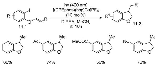
**Scheme 11.** Cu<sup>I</sup> photocatalyzed preparation of dihydrobenzofurans.
